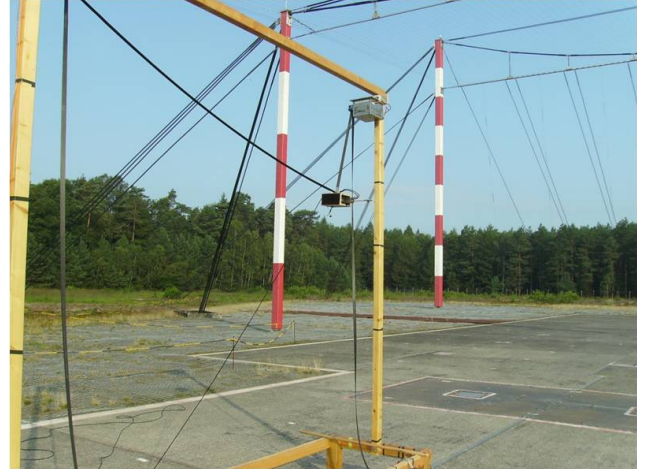
Fig. 2. Measurement setup in the DIES EMP simulator Munster. The actuators are mounted on a mobile wooden frame.
