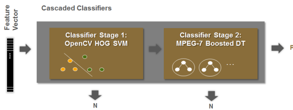
Fig. 1. Our cascaded classifiers try to reach high detection rates with the HOG-SVM in the first stage, and a second stage which focused on the avoidance of false detections, using MPEG-7 features and a boosted decision tree.
