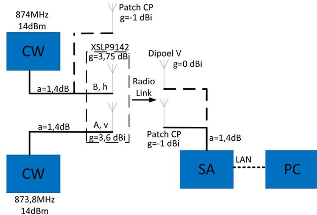
**Figure 2.** Measurement and test setup for the indoor radio channel modeling and the circular polarized patch antenna. (SA = spectrum analyser, CW = carrier wave generator).
