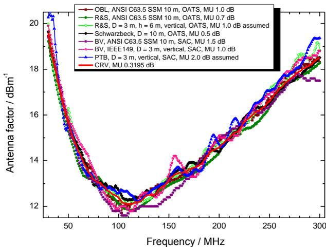
**Figure 2.** Results of intercomparison for SB VHBB9124 with BBAK9137.
