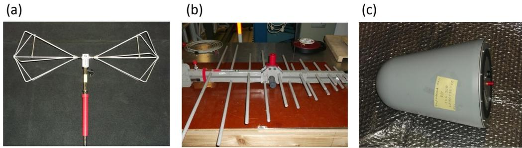
**Figure 1.** Antennas used as travelling standards. (a) SB VHBB9124 with BBAK9137, (b) AR<sup>®</sup> AT1000B and (c) R&S<sup>®</sup> HL050.
