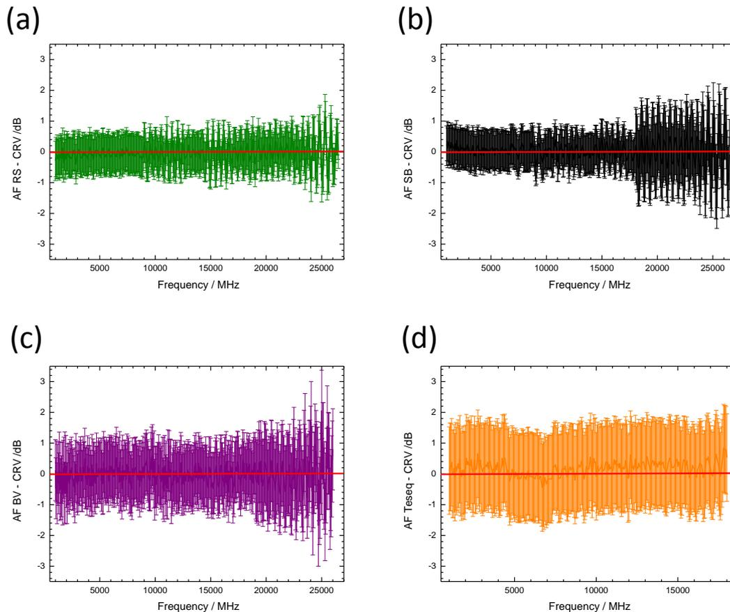
**Figure 7.** Results of intercomparison for the different participants and measurement constellations for Rohde & Schwarz<sup>®</sup> HL050. (a) R&S OATS 3 m vertical, (b) Schwarzbeck OATS 3 m, (c) BV IEEE 149 3 m vertical SAC, (d) Teseq 3 m SAC.
