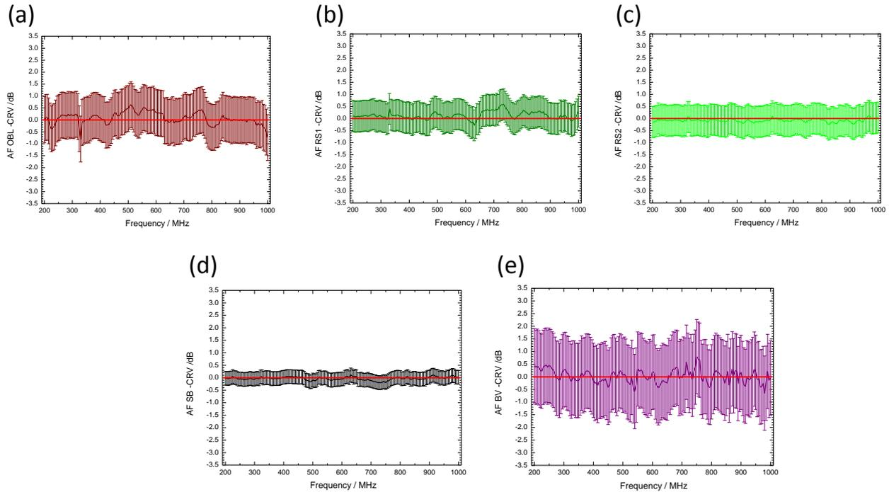
**Figure 5.** Results of intercomparison for the different participants and measurement constellations for AR<sup>®</sup> AT1000B. (a) OBL ANSI C63.5 SSM 10 m OATS, (b) R&S ANSI C63.5 SSM 10 m OATS, (c) R&S 3 m vertical OATS, (d) SB 10 m OATS, (e) BV ANSI C63.5 SSM 10 m SAC.
