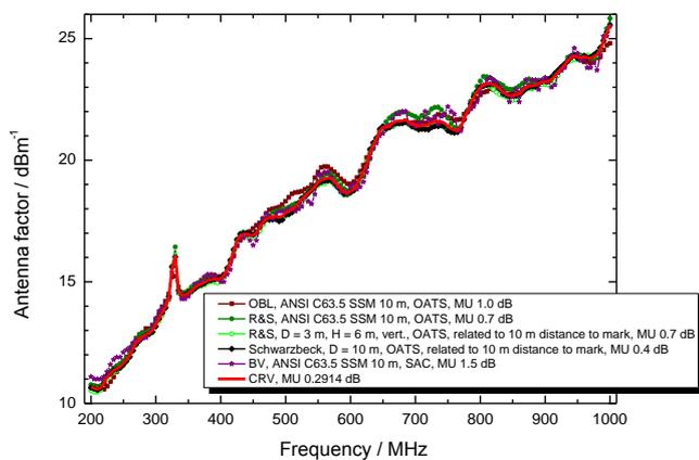
**Figure 4.** Results of intercomparison for AR<sup>®</sup> AT1000B.
