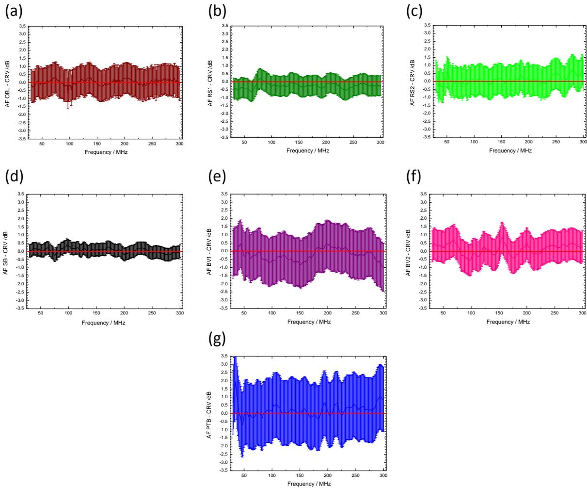
**Figure 3.** Results of intercomparison for the different participants and measurement constellations for SB VHBB9124 with BBAK9137 (a) OBL ANSI C63.5 SSM 10 m OATS, (b) R&S ANSI C63.5 SSM 10 m OATS, (c) R&S 3 m vertical OATS, (d) SB 10 m OATS, (e) BV ANSI C63.5 SSM 10 m SAC, (f) BV IEEE149 3 m vertical SAC, and (g) PTB 3 m vertical SAC.
