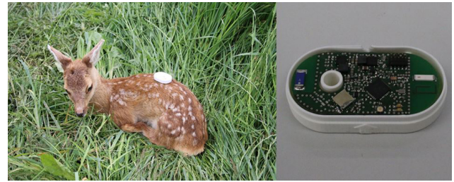
Figure 2. Marked fawn dummy and realized GPS-UHF-transponder.
