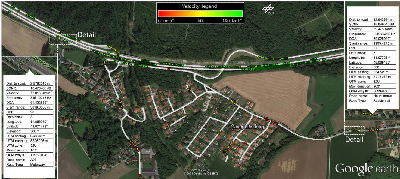
**Figure 7.** Results from the flight campaign over the Greifenberg area. Google Earth image overlaid with radar detections and their corresponding velocity estimations after using the road information. The cars (triangles) were automatically detected and their parameters were estimated using the proposed processor. The considered roads from the OSM database are shown in white.
