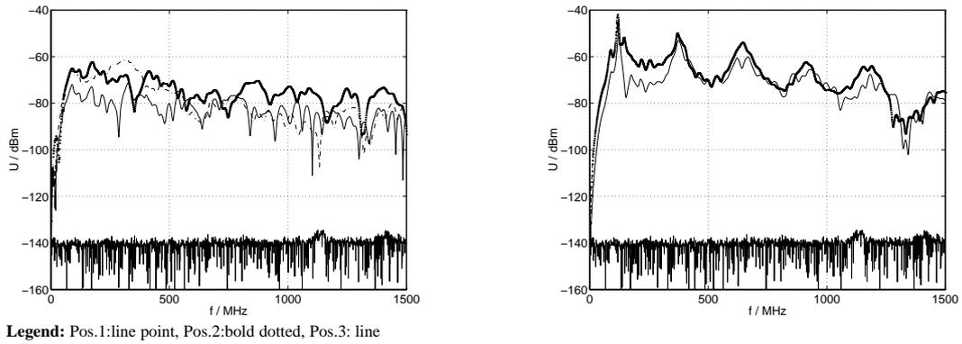
Fig. 3. Voltages of the 3 cable setups: Left: Loop antenna, perimeter = 1 m, Right: Monopole, length = 0.57 m.
