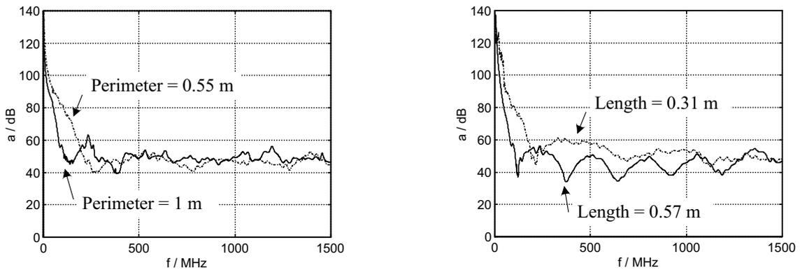
Fig. 4. Screening attenuation  $a_s$ : Left: Loop antenna, Right: Monopole.
