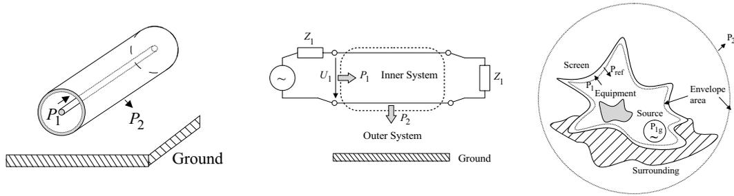
Fig. 1. Left: Coaxial cable. Middle: Equivalent circuit. Right: General screening attenuation.
