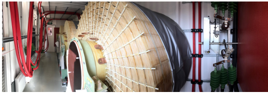
Figure 19. A look inside one of the test containers. In the foreground, some taps can be seen on one of the man-sized air coils. Source: http://delta-energie.de (last access: 8 January 2025).
