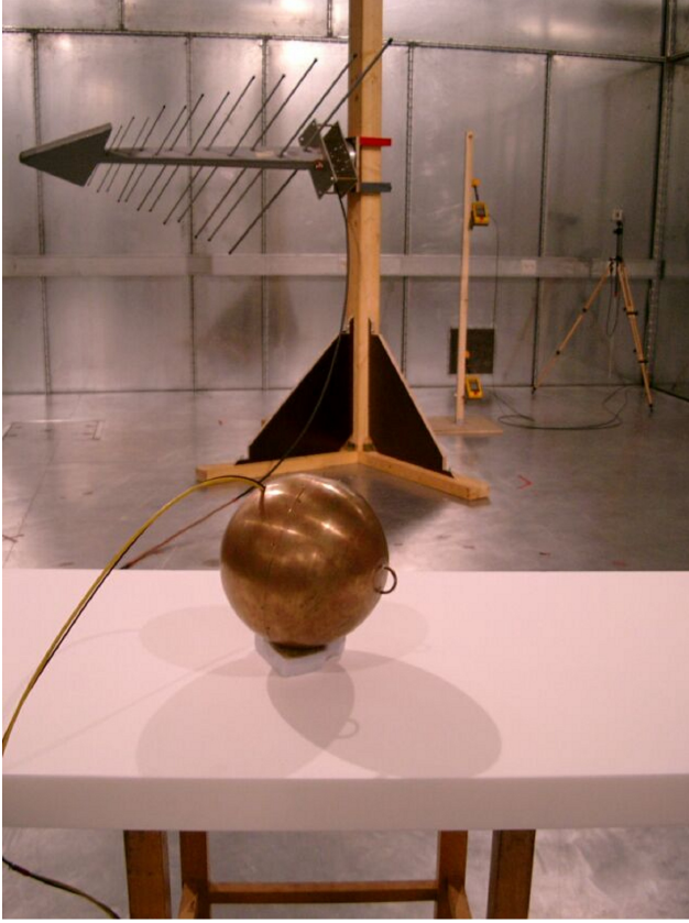
Fig. 3. Test setup in a Reverberation Chamber (TU Braunschweig). A logarithmic-periodic antenna (LPA) serves as transmitter, the surface current sensor is mounted on a sphere with 18 cm diameter (PTB Braunschweig). The metal sphere contains the electronics, only the fiber-optical link is penetrating the surface. The half-loop antenna can be seen in the front of the sphere at the right side. The transmitting LPA is not boresight at all.
