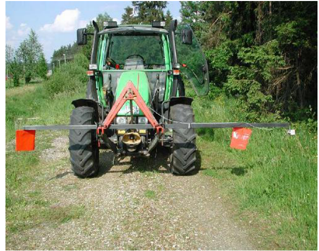
Fig. 9. Microwave sensor mounted at a tractor scanning the natural cover next to a dirt road.
