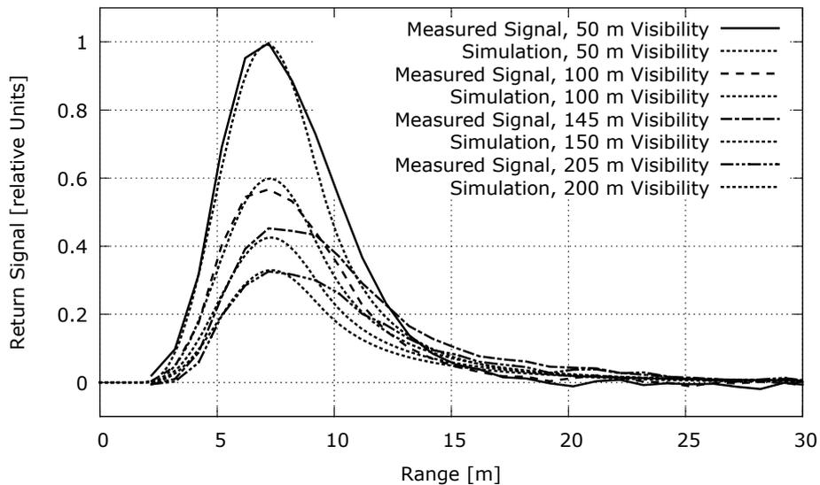
**Fig. 7.** Measured laser radar return signal in case of different visibility of 50 m, 100 m, 150 m and 200 m compared to numerically simulated return signals based on the theory presented in this paper. We assumed  $\alpha = \frac{3}{\text{Visibility}}$  and  $\beta = \frac{0.046}{\text{Visibility}} \cdot \text{sr}^{-1}$  as parameters for this simulation.
