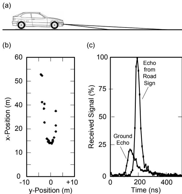
**Fig. 1.** (a) Beam configuration leading to detection of ground echo. (b) Typical spatial distribution ground echo detection, basis of shape-based ground echo classification. (c) Time domain classification of ground echo based on different time domain response of rigid targets (e.g. road signs, other cars etc.) and ground signal with different time domain response as shown by Issa (2007).
