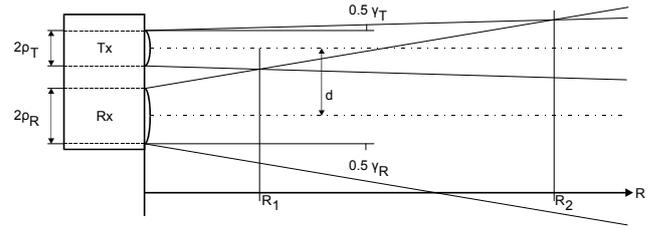
Fig. 2. Laser radar using a bistatic beam configuration.
