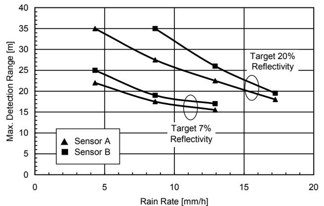
**Fig. 9.** Results of sensor tests using indoor rain simulator. The graphs show the maximum target detection range  $R_{MAX}$  as a function of rain rate for standard targets of 7% and 20% reflectivity and for sensors from two different manufacturers A and B.
